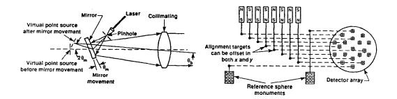
Fig. 2. Schematic of the Poisson Alignment Reference System
