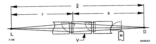
Fig. 1. Schematic illustration of the SLAC alignment system. T is one of 294 rectangular Fresnel lenses which focus laser light L to an image at the detector D. V is one of 60-cm diam. vacuum pipes, each 12 meters long which also serve to support the accelerator
