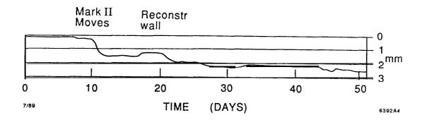
Fig. 4. Amplitude of Mark II dector settling on floor of SLC experimental pit. (Outboard levels are mounted in tunnels, inboard on piers in the pit supporting the final lenses.)
