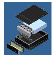
Figure 3: RSX-4 unit showing four detector locations. The ASPECT was equipped with 6 NaI[Tl] and 2 LaBr<sub>3</sub>:Ce scintillating detectors
