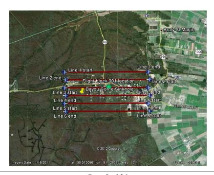
Figure 5: Flight planning lines for the chemical survey over Bayou Corne Sinkhole site
