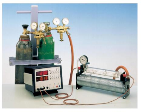
**Figure 3**: PHYWE experimental setup for demonstrating the Joule-Thomson effect.
