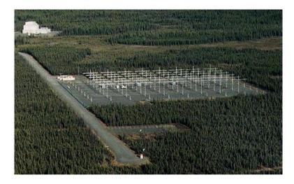
Above is an aerial view of the 48-antenna HAARP array. At top left is the Power Generation Building and Future Operations Center, to the left of the 48-Element HF Antenna Array is the Temporary Operations Center and the small structure at the bottom end of the runway is the Aircraft Alert Radar. The clearing above it is the Temporary Radiometer Pad.
