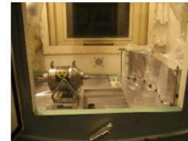
Figure 1: The set-up of the low dose rate experiment. Radiography camera and irradiation boxes housing the irradiation boards are mounted on an Aluminum frame that is positioned inside the heavy shielded box.
